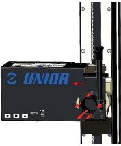
Unscrew top and bottom screws and disassembly motor protection and side protection from electric bike stand. Unscrew four screws from clamping head and remove it.
